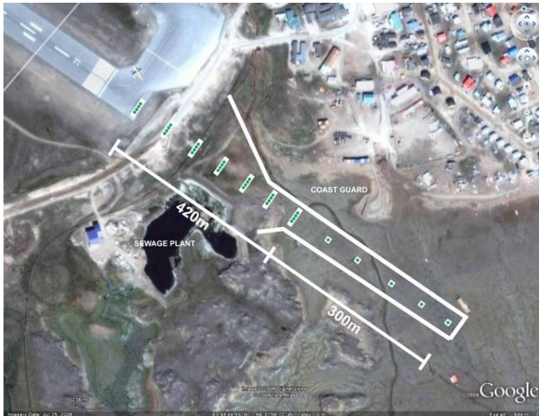
Figure W Graphic overlay showing location of proposed new runway approach lighting. 12 Red outline identifies landing beach.
