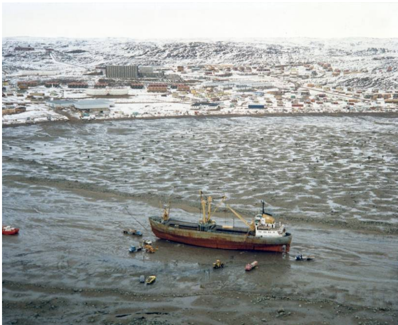
Figure H Arctic Viking being offloaded while aground on the Beach in Iqaluit (note the bouldery beach adjacent to the landing area which is kept cleared of boulders).
