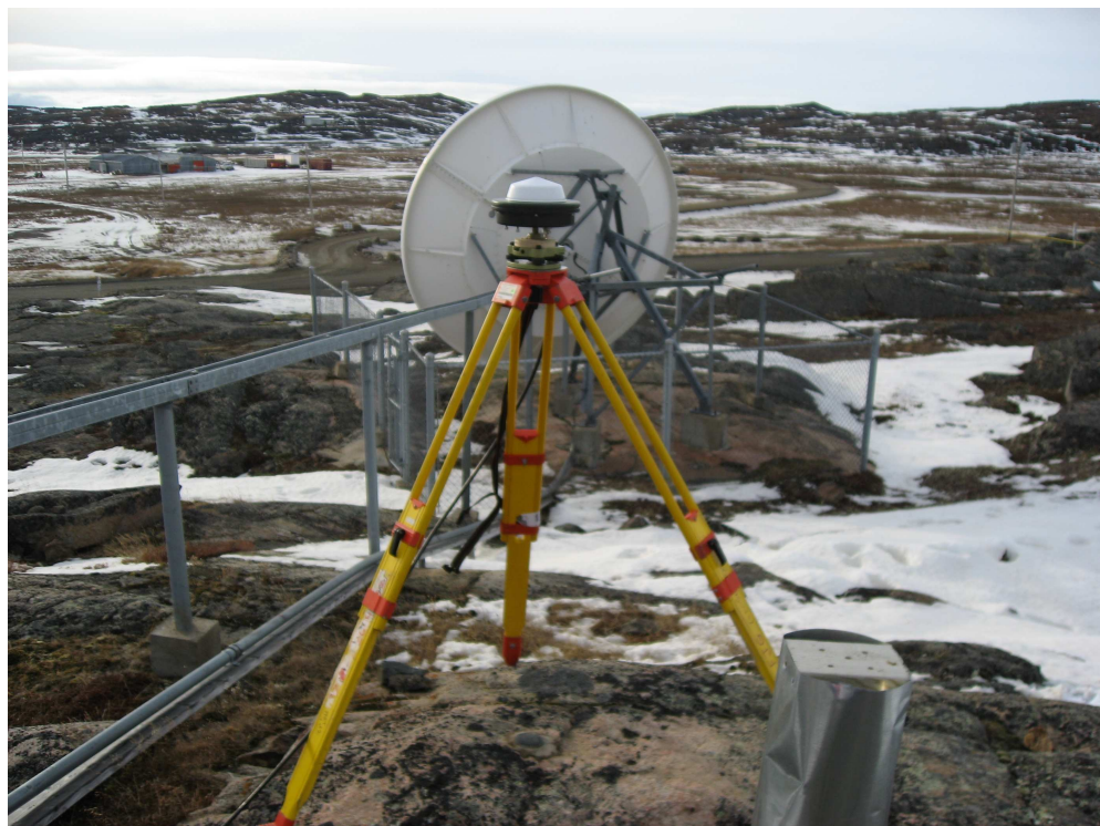
Figure 4.1: Static Survey - Antenna Setup
