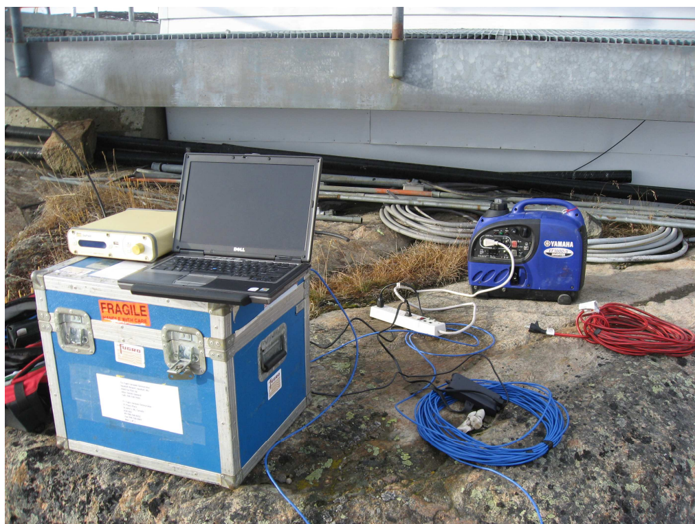
Figure 4.2: Static Survey – Starpack & Logging Laptop Setup
